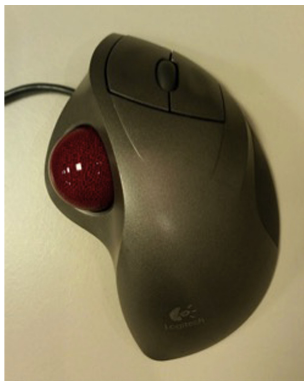
FIGURE 2: An ergonomic mouse with a track-ball feature. Note that this mouse positions the user's hand in less pronation than a standard device.
