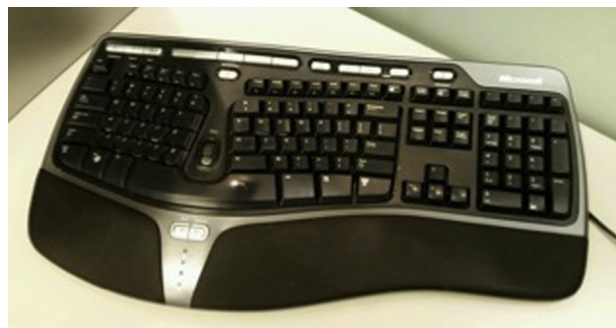
FIGURE 3: An ergonomic keyboard. Note that this keyboard positions the hands in less pronation, elevates the wrist to the level of the keys, and separates the hands. The wrists are placed in less ulnar deviation and the shoulders in less internal rotation.
